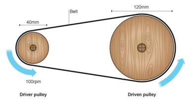
Output speed = Input speed ÷ Velocity ratio = 100 ÷ 3 = 33.3333..... rpm = <u>33.3 rpm</u> (to 1 d.p.)
