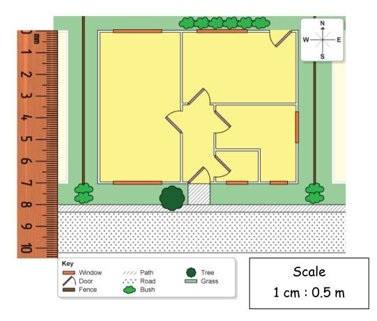
The scale on this plan drawing tells us that each centimetre on the drawing, represents 0.5 metres of the actual length of the building.
