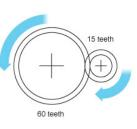
In **D&T** the main ratios you use are the **velocity ratio** in levers and pulley systems and the **gear ratio** when using gears. When you use ratios in D&T they are normally in the form of a calculation involving division.
