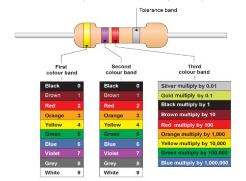
The first three bands on a resistor tell you the resistance.
